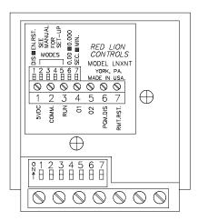
**Terminal 2** - "COMM." (common) Is the common line to which the sensor and other input commons are connected.
